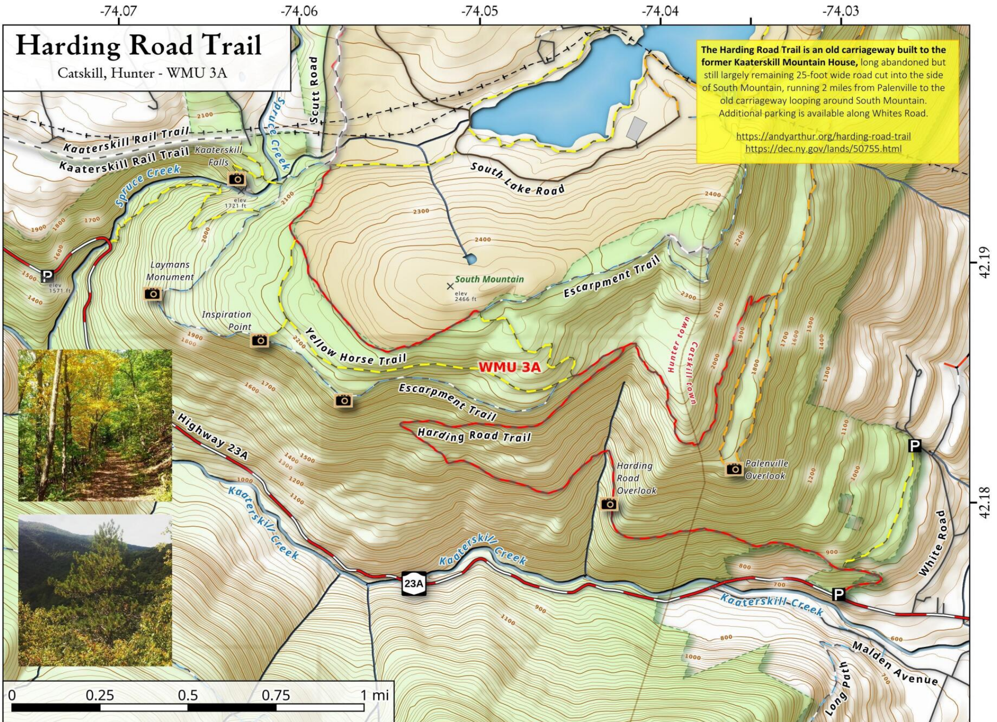
Harding Road Trail Map, October 2, 2019 by AndyArthur.org in QGIS 3.8.1-Zanzibar and Python. Street Map is Copyright © OpenStreetMap contributors, CC BY-SA. NYSDEC Data: LiDAR/DEM, Borders, ADK Wetlands, Trails, Assets. True North. 1 inch = 0.3 miles. Projection: NAD83 / UTM zone 18N. Coordinates: 0.01° latitude-longitude (WGS84). Contours are 20 feet. Map is centered on 42.1855,-74.0499.
